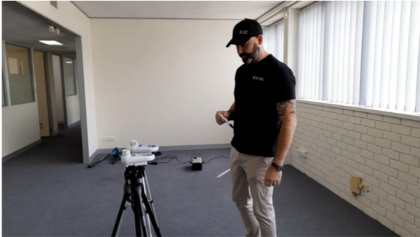
Figure 2: An Indoor Environmental Professional undertaking air sampling.
